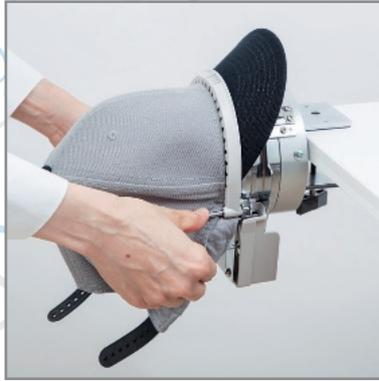
Sliding and ratchet frame fixing
