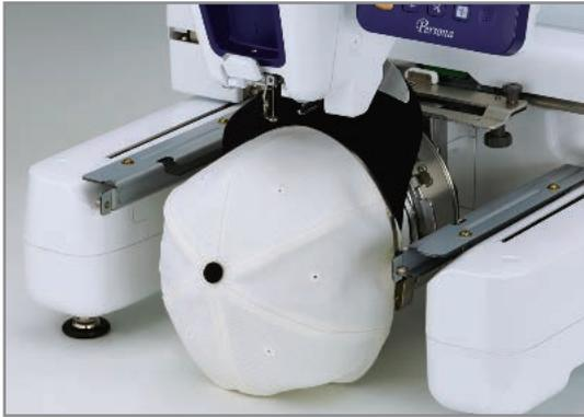
Set completed cap directly onto the machine
