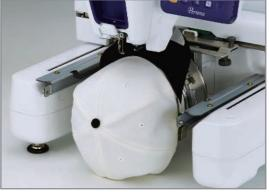
Set completed cap directly onto the machine
