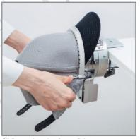
Sliding and ratchet frame fixing
