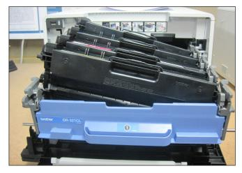
Replacing toner is a mess-free process. The toner cartridges lock into place on the drum unit. To replace toner, users open the access door, lift the cartridge assembly to eject it, then slide a new one into place. The cartridge positions are colour-coded.
