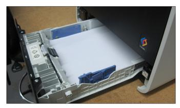
Adjusting the tray for different size media is straightforward, with length and width guides that move in sync.
