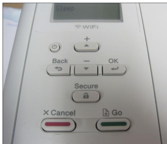
The HL-L8250CDN's control panel features eight hard keys (Go, Cancel and Secure for releasing secure print jobs, back cancel, power and up and down navigation keys) and a two-line, 32-character LCD display. The menu system is logically organized and easy to navigate.
