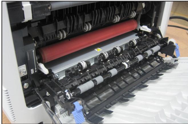
Misfeed locations are highly accessible. If misfeeds are removed from the rear, as illustrated here, the device may need to be turned around if placed against a wall or partition.
